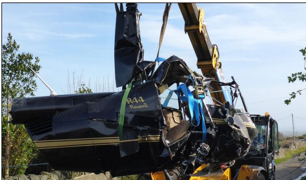
Photo No. 2: Damage to helicopter (photograph taken during wreckage recovery)
