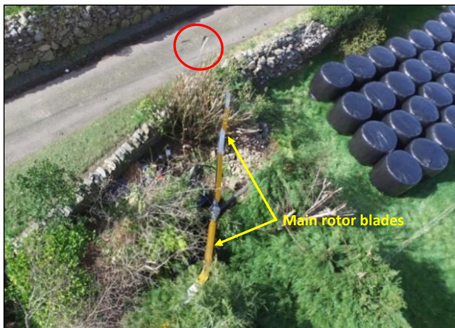
Photo No. 4: Aerial image showing damage to road surface (circled), with helicopter in dense trees/shrubs (main rotor blades annotated)
